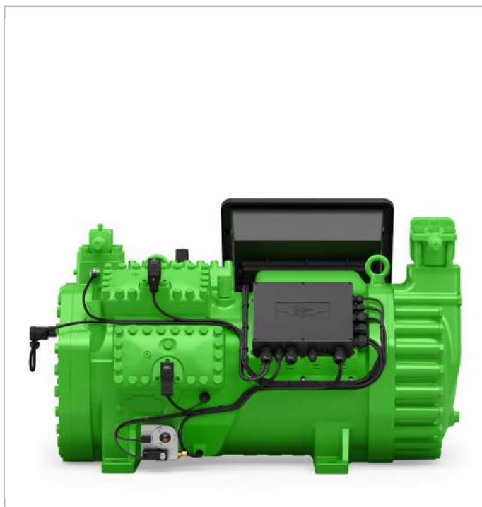
Fig. 12: Example equipment of a 8-cylinder compressor with CM-RC-02 compressor module, discharge gas temperature sensor, pressure transmitters, oil heater, CRII capacity control, differential oil pressure switch and OLM-IQ oil level controller.
