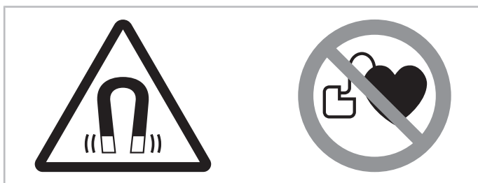
Fig. 16: Warning and prohibition signs on a compressor with permanent magnet motor
