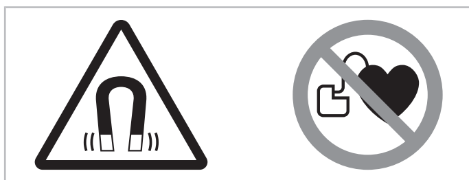
Fig. 12: Warning and prohibition signs on a compressor with LSPM motor
