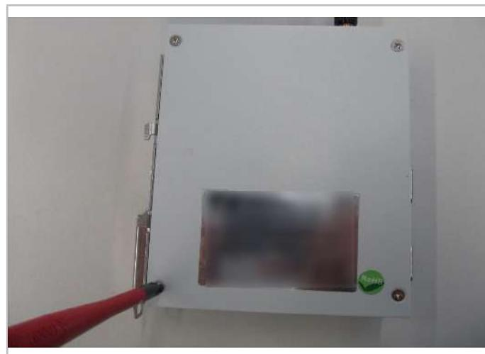
Fig. 17: Open the gateway housing with a screwdriver.
