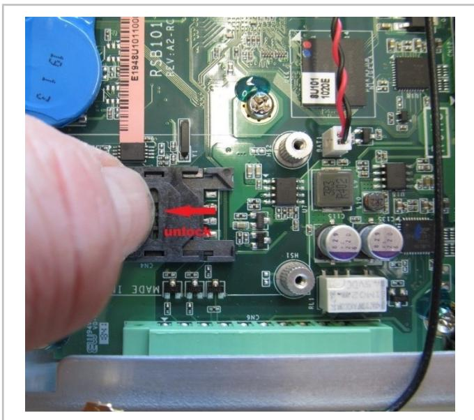
Fig. 21: Unlock the SIM card holder.
