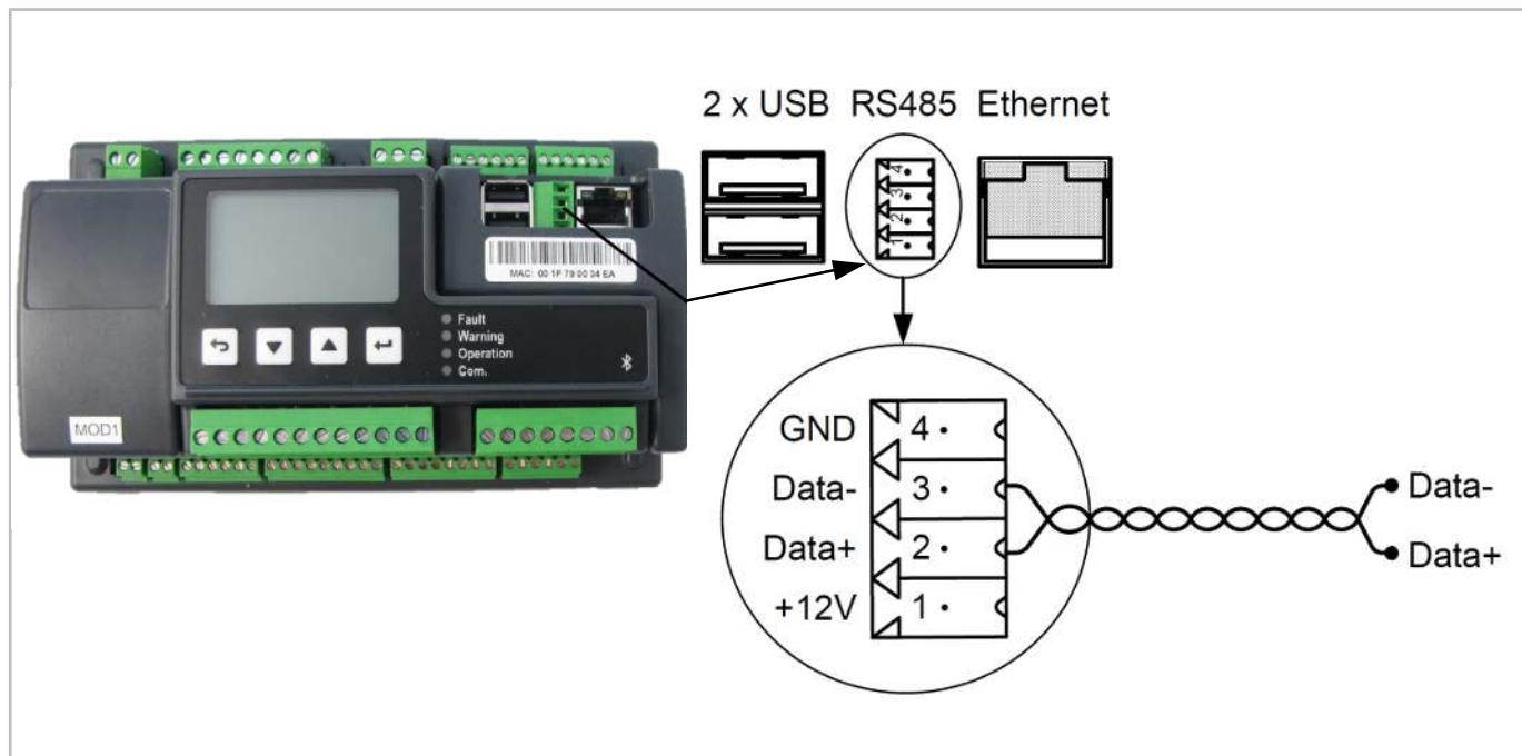
Fig. 15: Modbus connection at ECOSTAR controller
