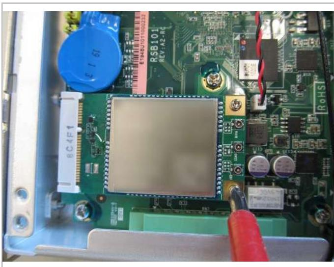
Fig. 19: Open the screws on the GSM module.
