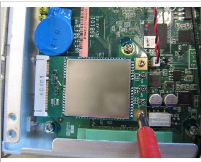
Fig. 19: Open the screws on the GSM module.
