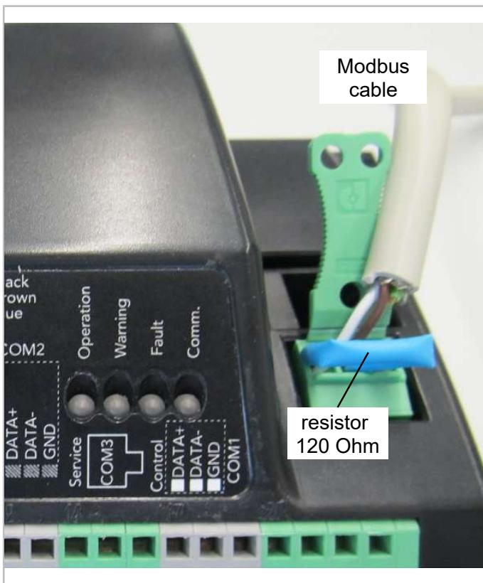
Fig. 10: Modbus connection on SE-i1
