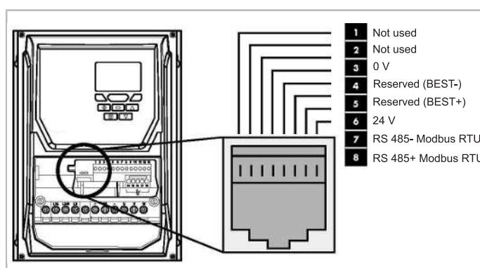
Fig. 14: Connect the FI to a PC via the BEST interface converter and the RJ45 adapter cable marked in blue.
