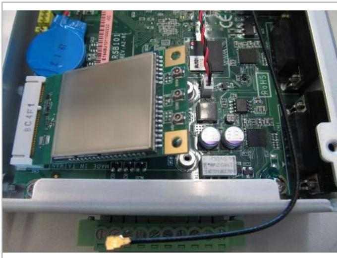
Fig. 20: Remove the GSM module.
