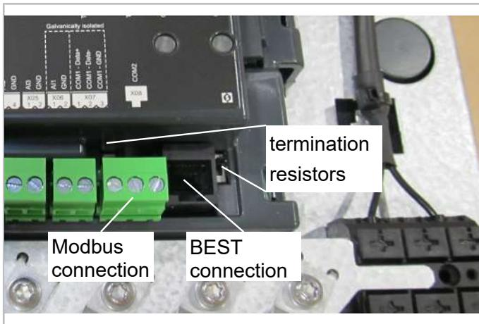
Fig. 11: Modbus/BEST connection at CSV compressor
