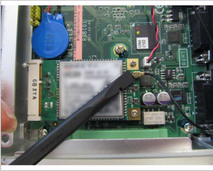
Fig. 18: Remove the antenna cable from the GSM module.
