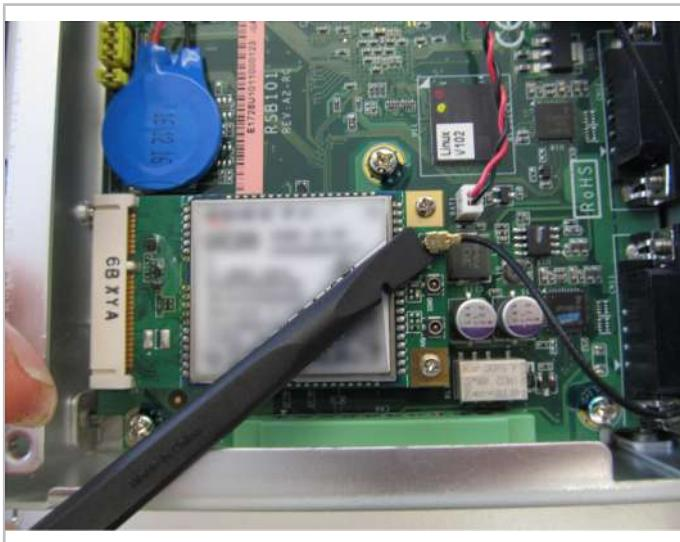
Fig. 18: Remove the antenna cable from the GSM module.
