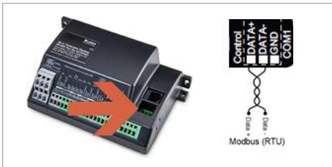
Fig. 23: Terminals of the Modbus interface of the SE-i1.
