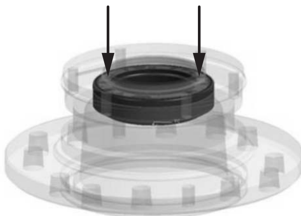
Fig. 1 Sealing cover with stationary ring
