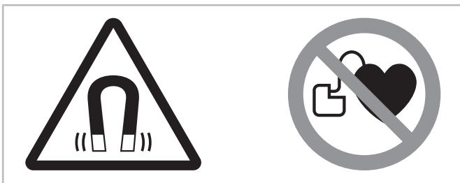
Fig. 14: Warning and prohibition signs on a compressor with permanent magnet motor
