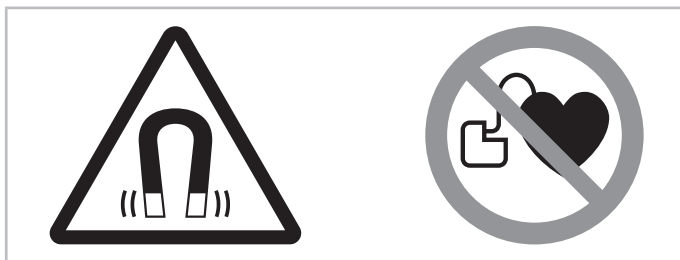
Fig. 11: Warning and prohibition signs on a compressor with permanent magnet motor
