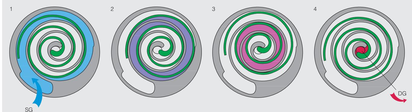
The moving spiral rolls within the stationary spiral in an orbiting way. The spirals contact each other at both flanks. They enclose several compression chambers which travel from outside to inside (see picture). The chamber volume is steadily decreasing. Thereby gas is taken in at the suction side and is compressed by volume reduction.
