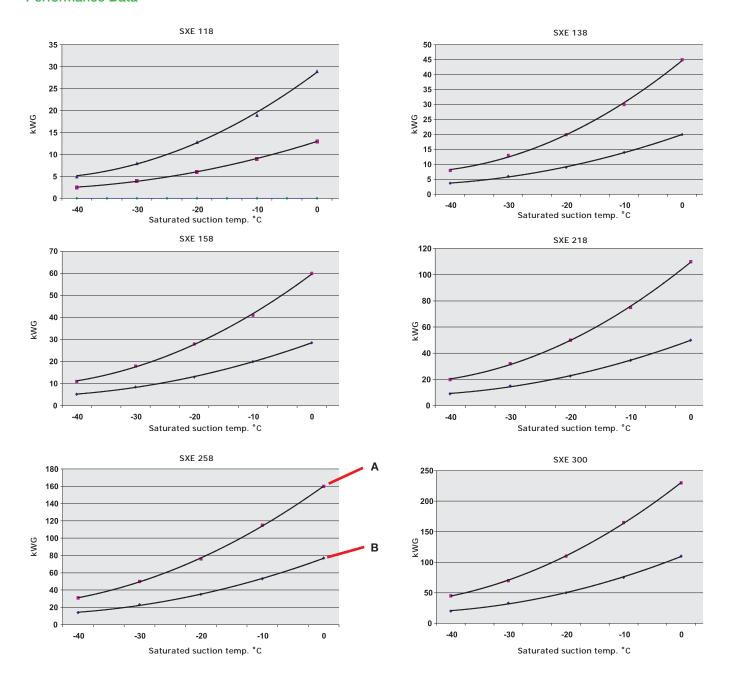
To select a suction accumulator, plot the operating point on the graph so it falls between the upper and lower limit lines.
