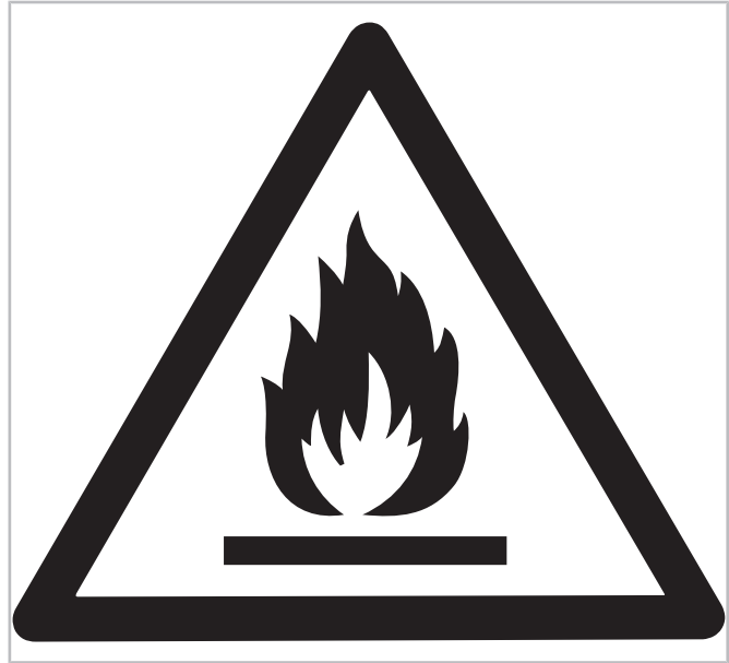
Fig. 1: Hazard symbol "Attention Risk of Fire" (ISO7010 W021)
