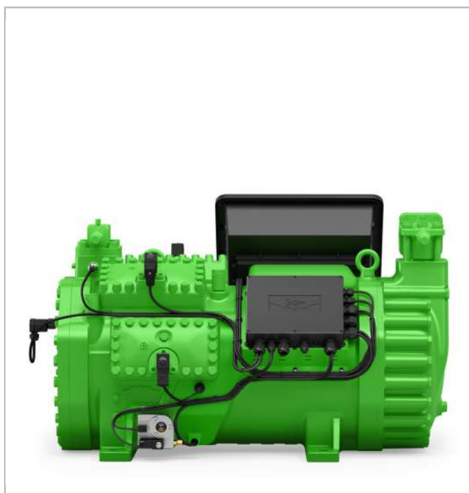
Fig. 11: Example equipment of a 8-cylinder compressor with CM-RC-02 compressor module, discharge gas temperature sensor, pressure transmitters, oil heater, CRII capacity control, differential oil pressure switch and OLM-IQ oil level controller.
